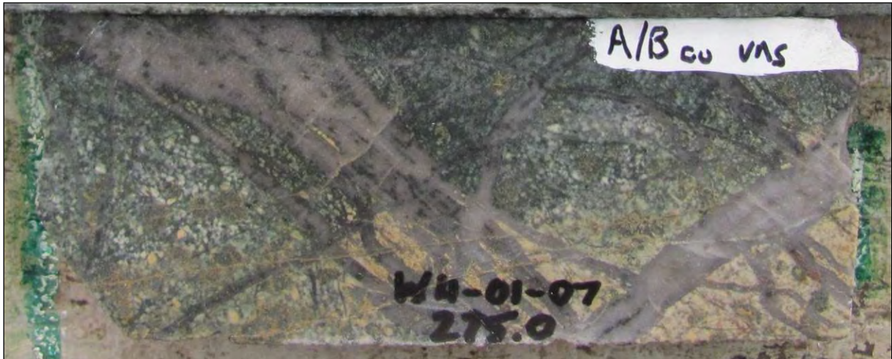
Figure 7-10 Photo of chlorite-sericite (+calcite) alteration overprinting potassic – magnetite alteration in a zone of quartz vein stockwork, subsequently cut by later Dpy veinlets with sericitic and iron-carbonate halos (Whistler Deposit) (Source: MMTS, 2016)
