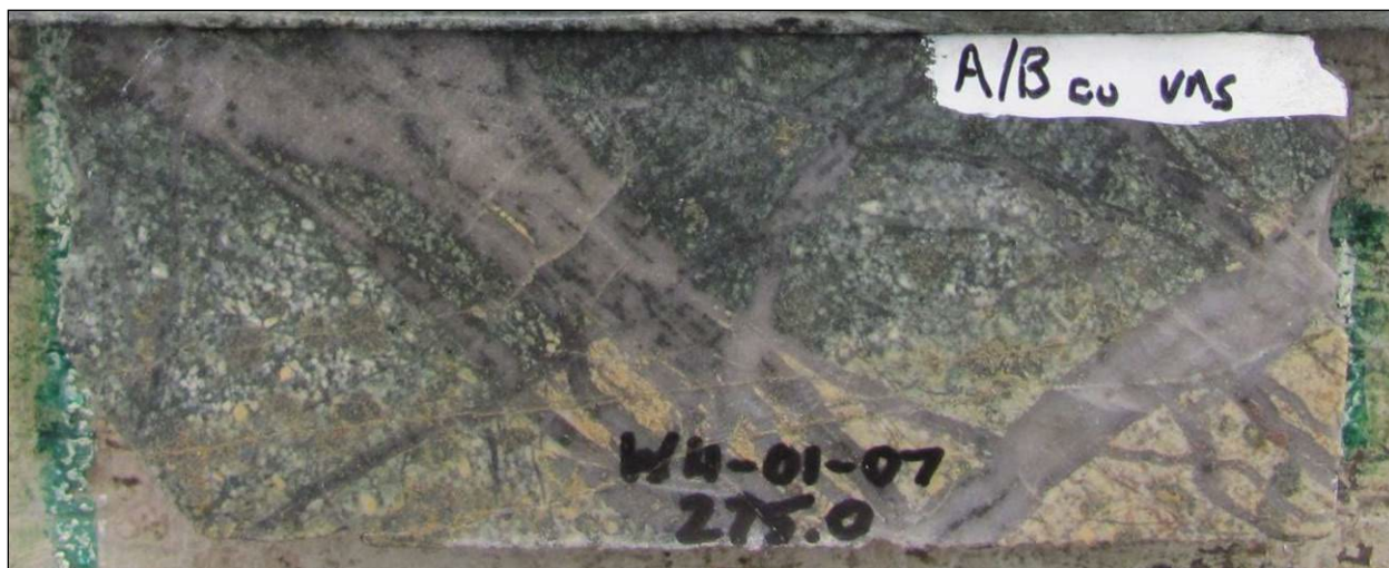
Figure 7-11 Photo of chlorite-sericite (+calcite) alteration overprinting potassic – magnetite alteration in a zone of quartz vein stockwork, subsequently cut by later Dpy veinlets with sericitic and iron-carbonate halos (Whistler Deposit)
