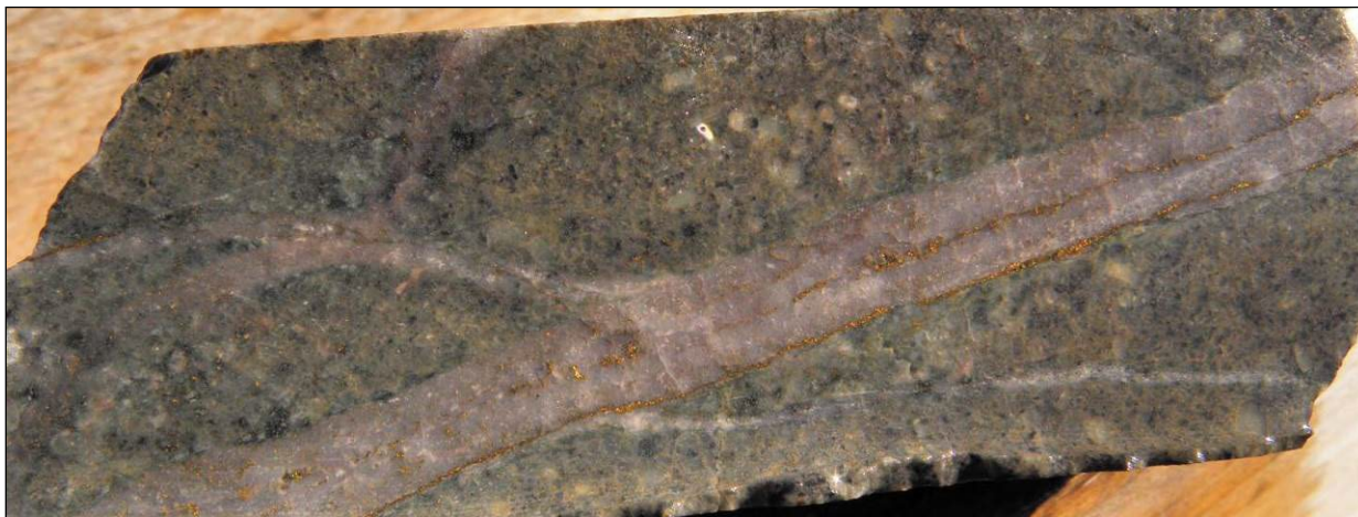
Figure 7-10 Photo of a classic B-style quartz vein with a chalcopyrite-filled centre-line cutting an irregular, wormy A-style quartz vein (Whistler Deposit, WH 08-08, ~123.0m)
