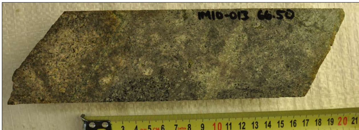
Figure 7-19 Photo of monzonite-matrix intrusive breccia with patchy albite alteration, silicification and disseminated chalcopyrite
