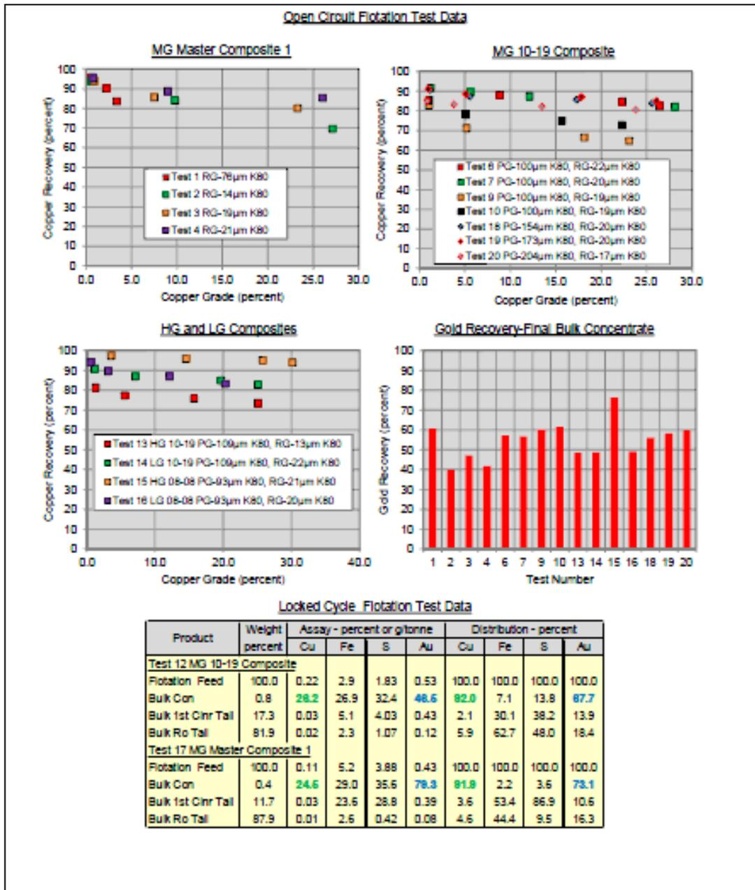
Figure 10-2 Flotation Test Results (MMTS, 2015)
