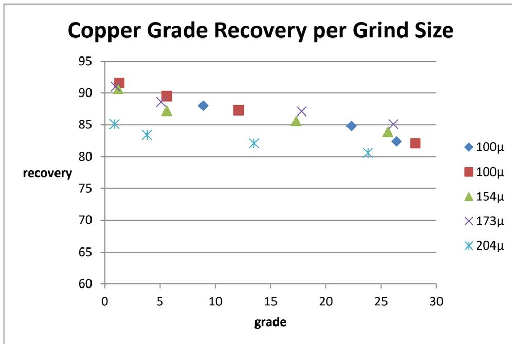
Figure 10-3 Copper Grade Recovery (MMTS, 2015)
