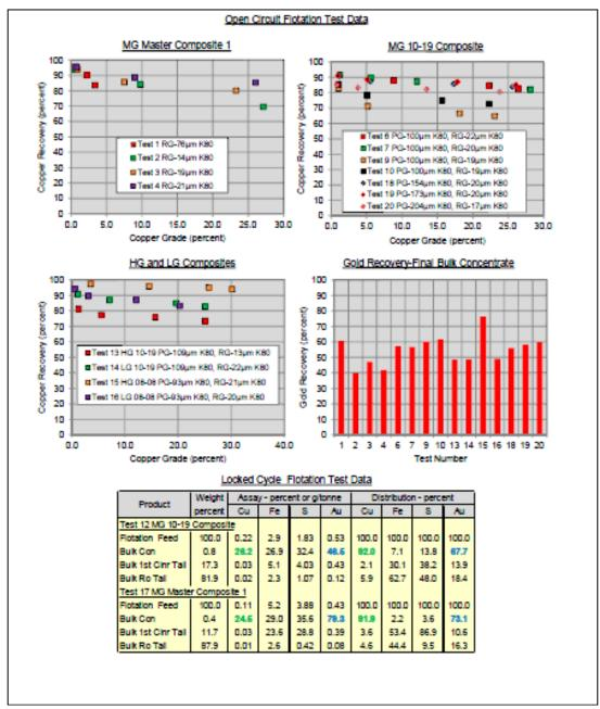
Figure 10-2 Flotation Test Results (MMTS, 2015)
