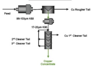
Note: A variable number of cleaning stages were used over the locked cycle tests. In some tests only two stages were required, in others three.
