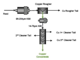
Notes: a) A variable number of cleaning stages were used over the cleaning tests. In some tests only two stages were required, in others three.
